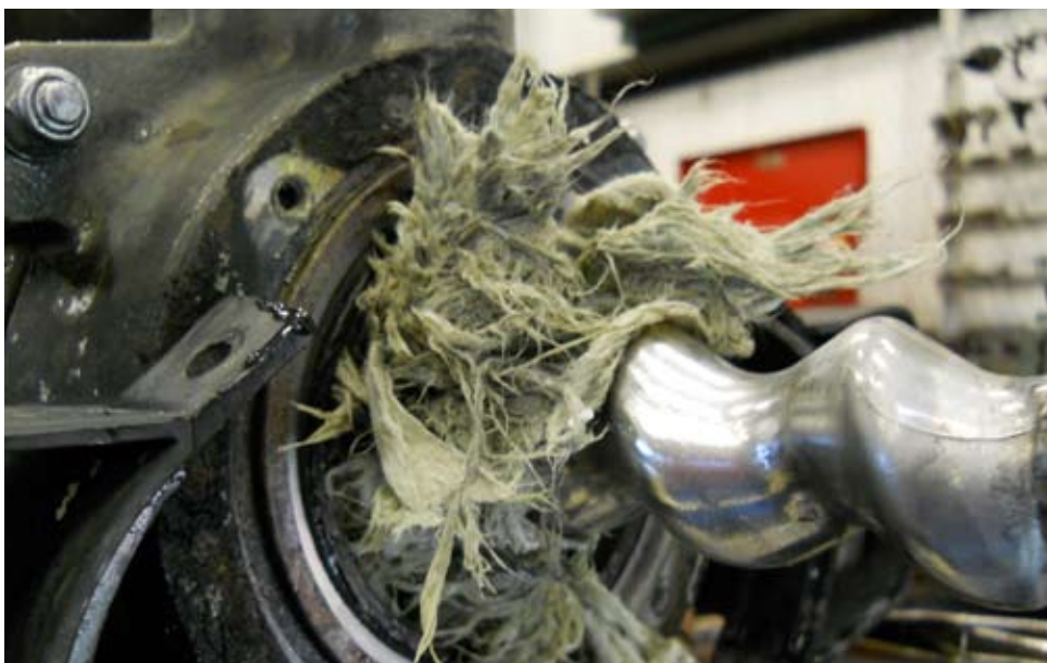
A grinder pump clogged by "flushable wipes" wrapped around the motor.
